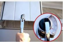
Our aluminum alloy code 6061/T6,hardness achieved 15HW.The wind load capability is base on the aluminum hardness
