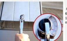
Our aluminum alloy code 6061/T6, hardness achieved 15HW.The wind load capability is base on the aluminum hardness
