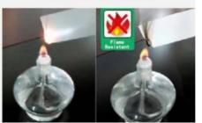
Cover:High quality double PVC-coated polyesster cextile,100% waterproof, flame retardant,UV resistant,tear resistant, self-cleaning ability,etc. Roof cover: 850g/sqm white PVC or 950g/sqm transparent PVC. Side wall: Transparent tempered glass wall.
