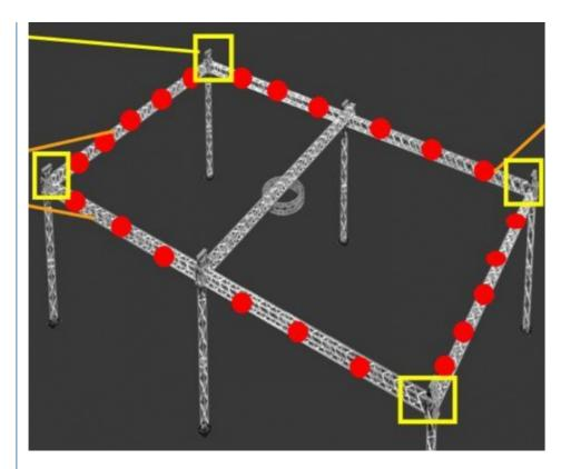
According to the calculation of the marks on the comprehensive diagram, 5 pieces of cloth (1.5 meters wide) are needed at 18 meters wide, and the middle distance of each cloth is 2.2 meters, and the middle distance of each cloth is 22 meters, and 6 pieces of cloth are needed, and the middle blank space of each cloth is 2.28 meters.
