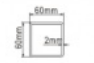
Eave Purlin, Gable pole, Ridge Purlin Intermediate Purlin 屋檐梁、横面横梁、屋脊梁 屋面方管
